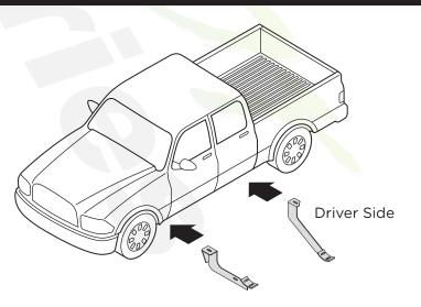
**4.** Install Front Mount Bracket by using one (1) Cab Mount Bolt.
