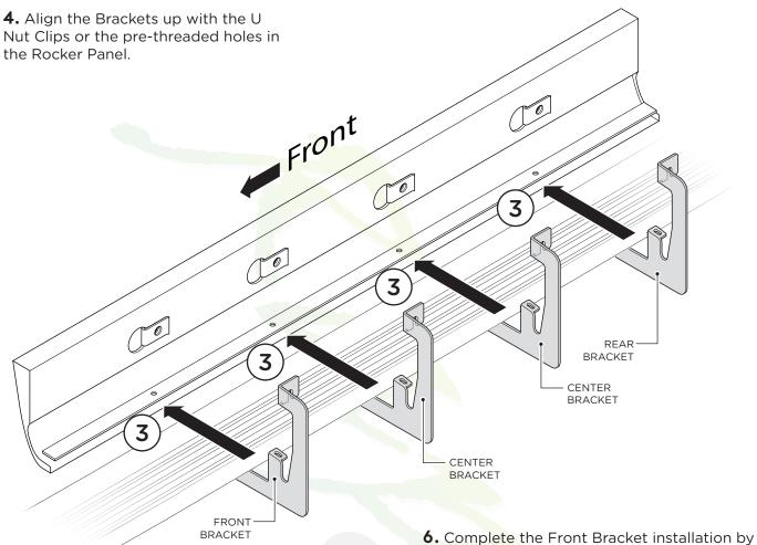
**5.** Fasten lower portion of the Front Bracket using one (1) M8 x 30MM Hex Head Bolt, one (1) M8 Lock Washer, one (1) M 8 Flat Washer, one (1) Weld Support and one (1) M8 Flange Lock Nut. Repeat for Center and Rear Bracket.
