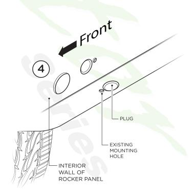
**5.** Remove the (2) plastic plugs from all (3) mounting locations in the rocker panel. Front Center and Rear. Insert M8 U Nut Clips so that the threads are on the inside of the rocker panel.
