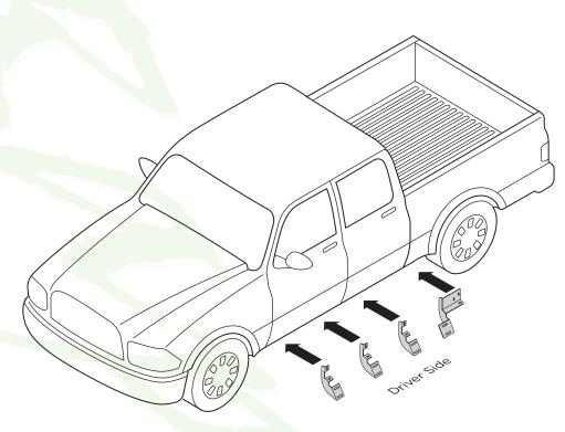
**4.** Existing mounting holes are located on the interior wall of the rocker panel. These mounting holes will be used per the following instruction.
