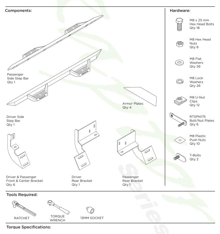
For Rocker Panel Mount Installations M8 through M12 bolts and nuts are set to 15-20 ft lbs.
