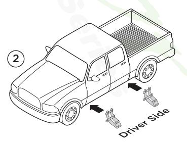
**3.** Existing mounting studs are located on the interior wall of the rocker panel. These mounting studs will be used for the following instructions.
