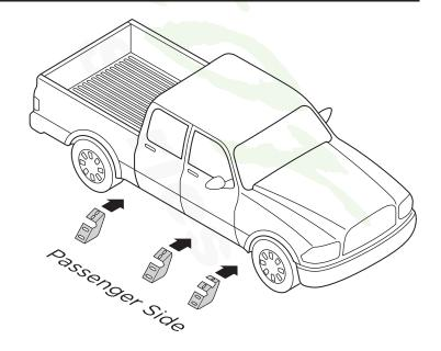
**4.** Align brackets with existing factory threaded holes in the rocker panel (4a). These holes may have black plugs in them that will need to be removed before installation. Fasten each bracket to the rocker panel using two (2) M8 x 30mm Hex Head Bolts, two (2) M8 Lock Washers and two (2) M8 Flat Washers (4b) per bracket.
