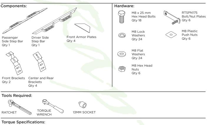
For Rocker Panel Mount Installations M8 through M12 bolts and nuts are set to 15-20 ft lbs.
