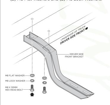
**3.** Fasten the top portion of the Driver Side Center Bracket by using (2) M8 x 30MM Hex Head Bolts, (2) M8 Flat Washers and (2) M8 Lock Washers.
