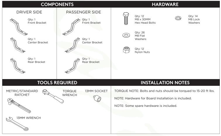
Remove all contents from the package and check brackets for any damage. Also, verify that all components and hardware listed above are included before you begin installation.
