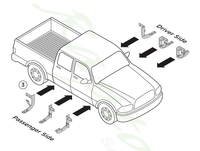
**4.** If threaded inserts already exist in Rocker Panel holes, fasten the top portion of the bracket by using (2) M8 x 30MM Head Head Bolts, (2) M8 Flat Washers and (2) M8 Lock Washers.
