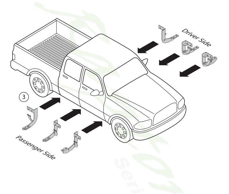
4. If threaded inserts already exist in Rocker Panel holes, fasten the top portion of the bracket by using (2) M8 x 30MM Head Head Bolts, (2) M8 Flat Washers and (2) M8 Lock Washers.
