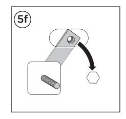
**6.** Fasten the bracket to the bolt side of the M8 Bolt + M8 Nut Plate by using (1) M8 Flat Washer, (1) M8 Lock Washer and (1) M8 Hex Head Nut.
