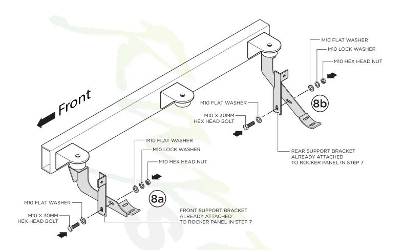
9. Place the Rubber Gaskets onto the Bracket Cradles. Then, place the Step Bar onto the Brackets.
