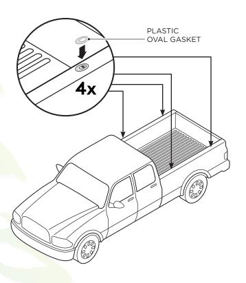
7. Fasten Rails to truck using one (1) 3/8" Flat Washer, one (1) 3/8" Lock Washer and one (1) 3/8" Hex Head Nut. DO NOT OVER TIGHTEN. Maximum tie down capacity perbed rail is 50lbs.
