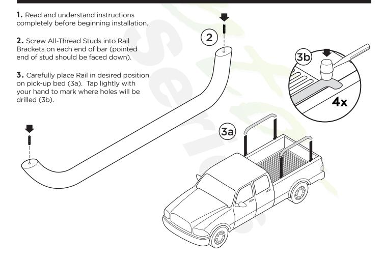
**4.** Drill 3/8" holes in top of Bed. Stud marks can be center punched so drill will not slip.
