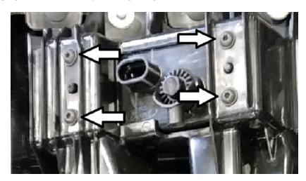
3. Mount the fog light to the fog light bracket by reusing the factory Torx screws. The brackets are driver/passenger specific.
