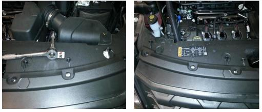
2. Remove the front grille and fascia from the vehicle. There will be several screws and plastic clips.
