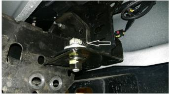
2. Remove the tow hook along with foam shield.
