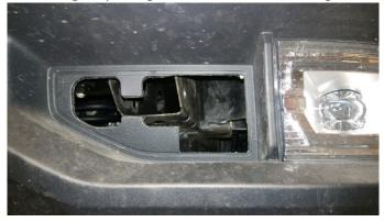
4. Slide the 5" tab w/the bolts through the top holes of the frame.
