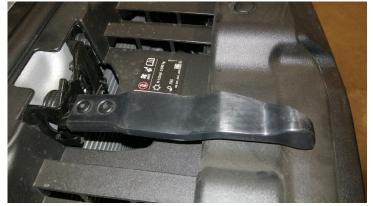
9. Remove the ten plastic clips holding the plastic shield located above the grille.
