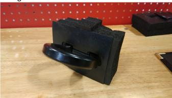
3. Cut a 2  $\frac{1}{2}$ " wide x 3" tall rectangle opening. This is for the mounting brackets.
