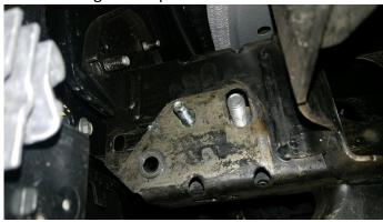
5. From the back side, slide the mounting bracket through the 2 %" x 3" opening and over the bolts. Use 3/8" and %" washers, lock washers and nuts to install.
