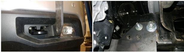
6. Reinstall the tow hooks. Use the factory tow hooks. If there are no tow hooks present, use ½" bolts. Also, at this time tighten the 18mm bolt that was loosened in step 1.
