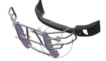
DETAIL C SCALE 1 : 1 NOTE: YOU'LL NEED TO MAKE A SLIT IN THE RUBBER GROMMET
