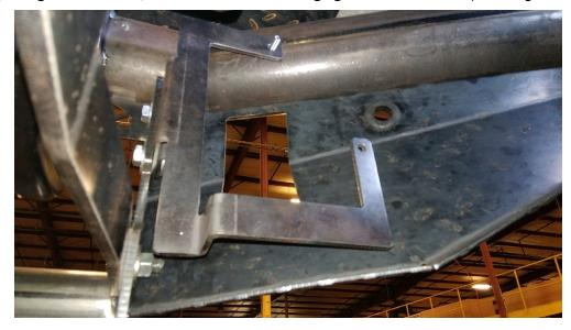
3. Second way is to mount the fog light, using ¼" hardware, to the brackets then mount to the bumper. (*Passenger light shown*).
