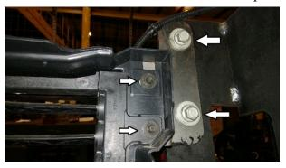
16. Hook up the sensor and fog light wires. Use the rubber grommets to install the sensors. You can run the wires through the square opening in the mounting brackets just below the top plate. **On the outer sensors, use the two pigtails.** Adjust the lights and sensors if needed.
