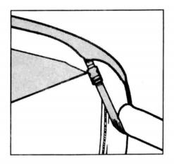
STEP THREE: LAY THE BACK OF THE BRIEF OVER THE MAIN BAR OF THE ROLL BAR AND PULL THE REAR CORNER STRAPS UNDER THE REAR ROLL BAR BRACE AND UP TO THE QUICK RELEASE BUCKLE. THREAD THE STRAP THROUGH THE QUICK RELEASE BUCKLE AS ILLUSTRATED. DO NOT TIGHTEN COMPLETE. REPEAT THE ABOVE INSTRUCTION ON THE OPPOSITE SIDE. NOW TIGHTEN BOTH SIDES COMPLETELY.
