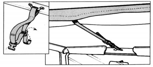
STEP FOUR: ADD THE FEMALE SIDE OF THE QUICK RELEASE BUCKLE (SUPPLIED WITH BRIEF) TO THE CENTER STRAP IN THE MIDDLE OF THE WINDSHIELD FRAME. PULL THE CENTER STRAP FORWARD AND THREAD THROUGH THE MALE SIDE OF THE QUICK RELEASE. TIGHTEN THE CENTER STRAP.
