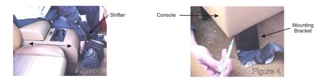
5) Once the position is marked, remove the Console from the vehicle and set on a clean working table.
