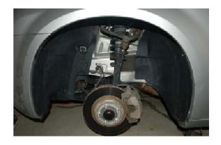
*Step 2*) Remove the factories wheel well clips, that secure the fender liner to the vehicle. To remove the clips, pop the inner tab out of the assembly first then remove the complete assembly by prying the outer edges of the clip.
