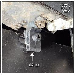
**IMAGE D** Position logoed flap MF84-LF/RF-BOT over top MF94-LF/RF-TOP holes. Assemble using SMWASH and HXBLT on logo-side and SMWASH and BLKNUT on tire-side of flap.
