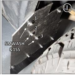
IMAGE J Place 1SP between flap and liner, then install SMWASH and 2SS into mount 4.
