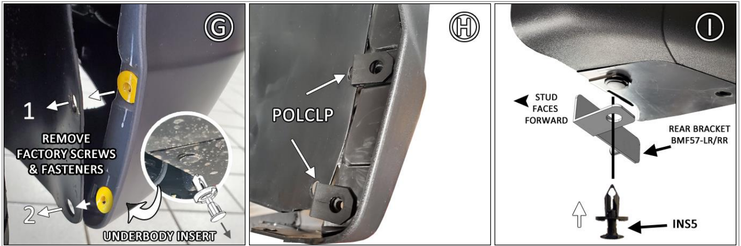
FIGURE J Place .25SP on the logo-side of mud flap against mounting points 1 and 2.
