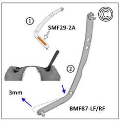
**FIGURE D/E** Position BMF87-LF/RF bracket behind mud flap. Place logo-side of mud flap facing rear of the vehicle against mounting points on liner and bracket. Use 1.5SS & SMWASH to fasten points 2 & 4. Use SSLNUT & SMWASH for mounting points 1 & 3. Ensure inner foam spacer contacts liner. Repeat Figure C as needed.
