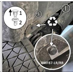
**FIGURE J** Place logo-side of mud flap facing rear of the vehicle against corresponding mounting points. Use 1.5SS & SMWASH to fasten points 1 - 3. Use SSLNUT and SMWASH for mount #4. Do not fully tighten.
