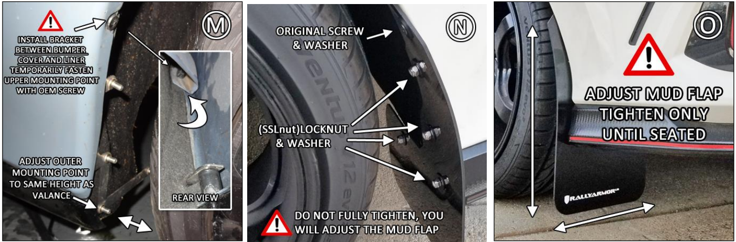
FIGURE O Align outer edge of the flap by making small angle adjustments to the flap then walk away to make sure it's even with the ground. Tighten all hardware only until seated against mud flap.
