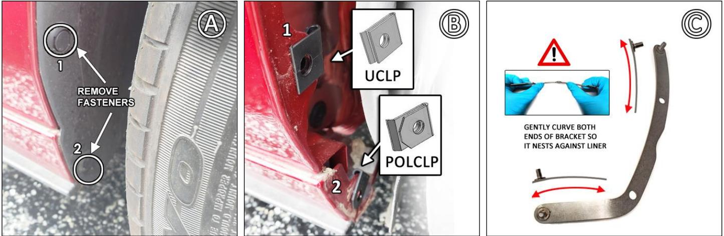
**FIGURE E** Place mud flap logo-side to the rear of the vehicle against mounting points on the bracket and liner. Pair WASHERS WASH & SCREWS 1SS to fasten mount 1 & 1.5SS and WASHER WASH for mount 2. Use a WASHER WASH & LOCK NUT SSLNUT for points 3 & 4. Do not fully tighten.
