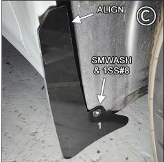
**FIGURE D** Align flap edge against fender edge. Clean area behind fender edge before adhering **15TAB 8.75"** from top of flap to center of **15TAB**. Adhesive side faces tire.
