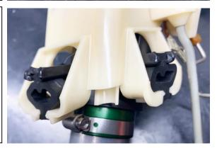
21. Locate the new fuel pump sock filter and the metal lock washer. Insert the sock onto the bottom of the pump. This installs only one way. NOTE: filter sock may differ than picture.
