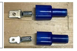
13. The OEM fuel pump wires use female spade terminals. Each of these terminals have tabs that lock into the holes of the male connectors. Depending on the force applied to the tabs when the terminals were removed, it is possible for them to be over bent. In this case, use a small pick to press the tab downwards (as shown in top picture).
