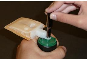
22. Slide the 2 sections of heat shrink over each BMW female spade terminal.
