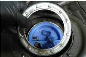
25. Connect the battery and turn the key to the ON position. Listen for the new fuel pump to confirm the electrical was performed properly and check for fuel leaks. If no leaks are found, start the vehicle. The engine may run rough for a few seconds until the air is bled from the system.
