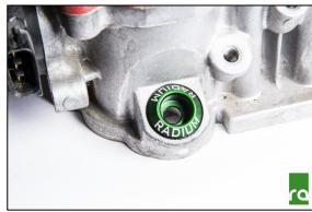
4. Radium Engineering injector seats for Toyota. 5. Radium Engineering injector seats shown for Mazda primary rail.  $5. \ Radium \ Engineering \ injector \ seats \ shown \ for \ Mazda \ secondary \ rail.$
