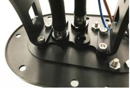
14. From the backside of the assembly, remove the two outer M5 bolts using a 3mm Allen hex wrench. Detach the collector box from the assembly, as shown.
