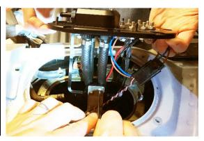
24. Continue to lower and rotate the assembly until the Radium collector box sits properly into the OEM gas tank baffle. Not visible, but shown is what the inside of the gas tank would look like.
