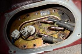
5. To detach the SAE quick disconnect lines, simply squeeze the locks and pull the fitting away from the metal tube. Reinstall the plastic lock to the fitting. To detach all other hoses, use pliers to release the spring clamps and pull the hoses off. Use a rag to clean up any spilled fuel.
