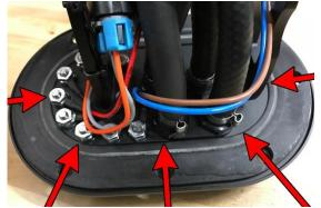
23. NOTE: The level sender cannot be attached until the hanger assembly is halfway installed into the gas tank. This step MUST be performed with 2 people (Installer#1 and Installer#2). First, remove the 2 small M4x0.7mm screws from the hanger bracket using a 2.5mm Allen hex wrench. Then, while outside the gas tank, plug in the connector with blue and brown wires to the level sender connector that was assembled in earlier steps.
