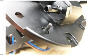
22. From the underside of the top plate, be sure that the OEM gasket is seated in the machined lip, as shown.
