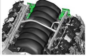
9. The 20-0232 fuel rail does not include plumbing. NOTE: Early LS1 engines (97-99) will require an aftermarket FPR to replace the regulator on the OEM rail.
