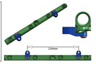
5. To secure the mounting feet to the rails, install the included split lock washer and M5 bolts (as shown).
