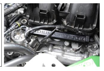
16. For 20-0111-00 or 20-0111-PK, use a short Phillips head screw driver to loosen the hose clamp on the fuel feed line, the one that was disconnected in step 5.
