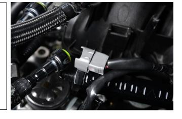
15. Orientate the #2 injector so that the electrical connector clears the OEM high pressure fuel pump.
