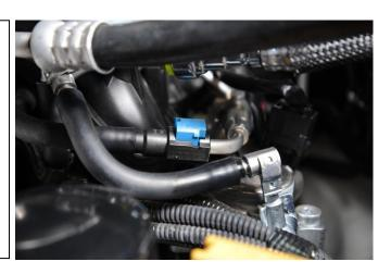
5. Use a fuel line release tool to detach the fuel feed hose from the fuel rail pipe.
