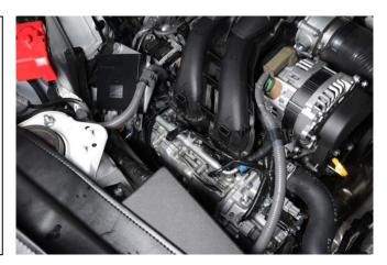
22. Unplug the electrical connectors for the two fuel injectors. Unlock the fuel cross-over hose by pulling out on the blue clip. Disconnect this hose from the fuel rail pipe.
