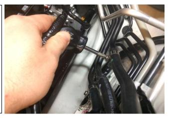
17. Find the PTFE hose included in 20-0111-00 or 20-0111-PK that has a 90 degree fitting on one end and no fitting on the other. Install the included hose clamp onto the end that does not have a fitting.
