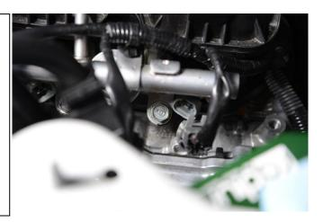
7. With fuel rail out of the car, remove the injectors.
