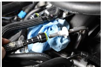
6. Unplug the electrical connectors on each fuel injector.
