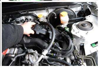
4. Locate the crossover fuel hose connection on the front of the LH fuel rail. The hose end fitting has a blue clip.
