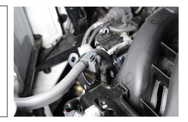
21. Remove the three M6 bolts holding the ECU to the brackets.
