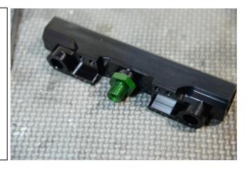
11. Place the crush washer from Step 9 on the adapter fitting then screw on the pulse damper. Tighten with a 7/8" or 22mm wrench.
