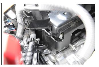
27. Before installing the metal cover, clip the ears off the injector connect (as performed in steps 13 and 14) for the rear injector connector on the RH side. This will allow the injector to rotate in place enough to clear the metal cover. NOTE: This is not required if the fuel rails were purchased after October 2018.
