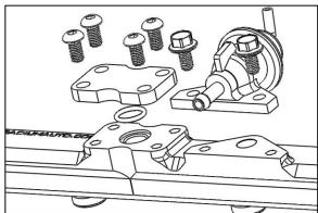
12. When mounted, the rear of the fuel rail will come close to contact with the OEM air control valve (notch if necessary). Install an 8AN ORB "port" plug fitting (such as Radium P/N: 14-0150) to the rear port if the OEM air control valve will remain in the vehicle.
