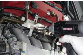
7. Using a 10mm socket wrench, remove the four M6 bolts that secure the two mounting brackets that attach the fuel rail to the intake manifold runners. These two brackets will be reused.
