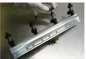
9. Gently pull each fuel injector from the OEM fuel rail. Inspect all O-rings and grommets for rips and tears and replace, if necessary. Lubricate the O-rings when reinstalling injectors into Radium fuel rail.
