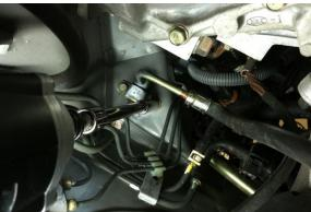
17. Remove and discard the Honda OEM soft rubber hose (shown) from the vehicle.
