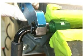
19. From underneath the vehicle, mate the inverted flare fittings. Route the PTFE hose upwards staying clear of hot and/or moving parts. Secure to the -6AN male fitting on the top port of the fuel rail.
