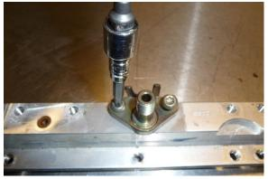
11. If the OEM banjo will NOT be reused, install the included block-off-plate, O-ring, and 4 button head screws, as shown. Lubricate the O-ring with clean engine oil.
