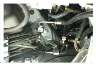
16. Using a 10mm socket wrench and extension, remove the two M6 bolts that secure the fuel feed line clamp to the chassis, as shown. These will not be reused.
