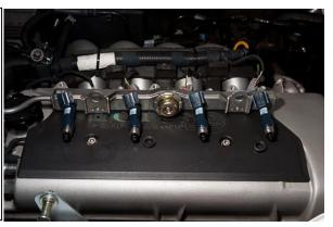
5. On the stock fuel rail, locate the fuel pulse damper. Gently pry up on the tabs that hold it in place.
