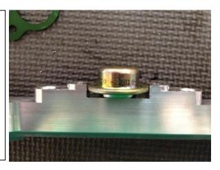
8. Use the included green anodized flat bracket to hold the damper in place. Secure with the two included M5 Allen bolts.
