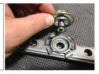
7. To prevent failure, lightly lubricate the o-ring on the damper and install into the center port on the Radium billet fuel rail.
