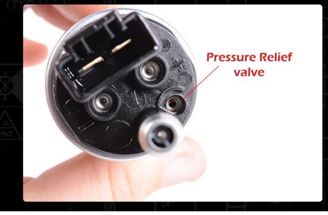
The pressure at which these values open is documented on the Fuel Pump Identification Page. Most open in the 87 psi range. When the value opens, fuel sprays out, relievieving the pump's internal pressure. When this happens, flow to the engine is reduced due to the flow lost through the pressure relief value.
