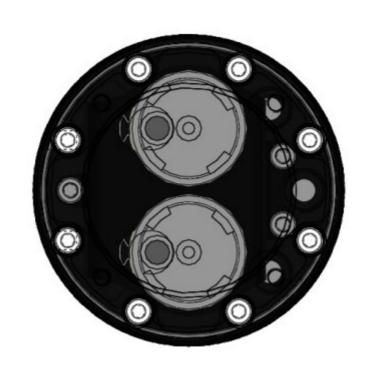
If a dual pump standard fuel surge tank MUST be mounted in horizontal configuration, it should be oriented as shown below, with the pumps side by side. This is not 100% optimal, but will work. In a situation like this, any sort of positive mounting angle will be very helpful to allow the surge tank to utilize its full volume as much as possible.
