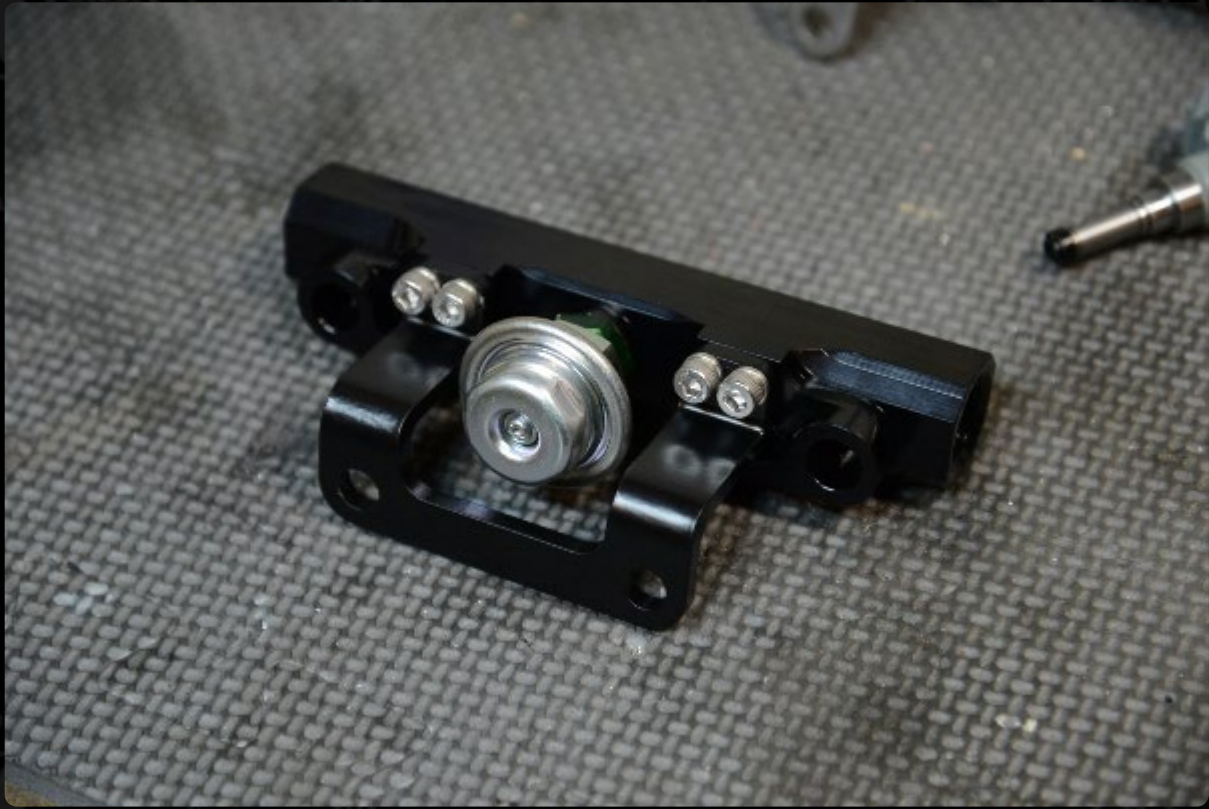
Radium Engineering FR-S/BRZ fuel rail with OEM fuel pulse damper mounting port
