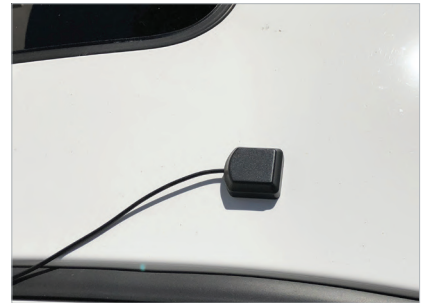
6. Route and mount the GPS antenna on the ROOF or TOP of vehicle, with a clear view of the sky.
