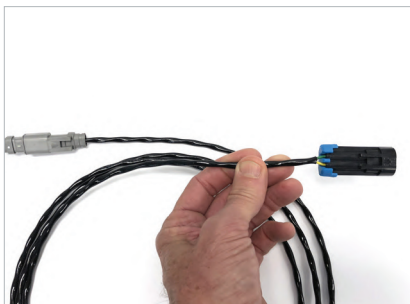
4. Connect the opposite end of the interface cable to the ECU. Connector varies based on ECU.
