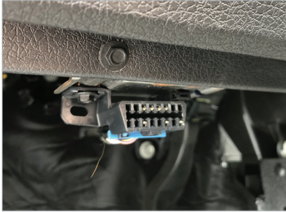
1. Locate the vehicles OBD2 connector.
