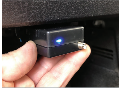
2. With vehicle power OFF, plug the CL2 into the OBD2 connector.
