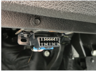
1. Connect the CL2 to the vehicles OBD2 port
