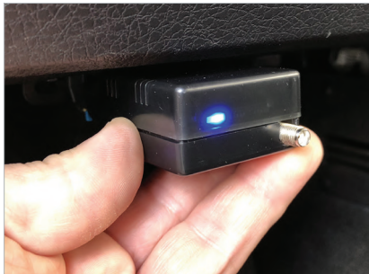
1. With vehicle power ON, the LED adjacent to the GPS antenna connector should glow BLUE.
