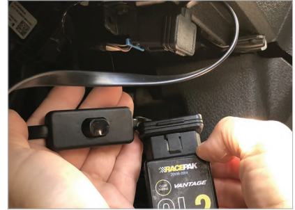
3. If the vehicles OBD2 connector places the CL2 in an undesirable location, the OBD2 extension cable can be utilized to relocate the CL2.
