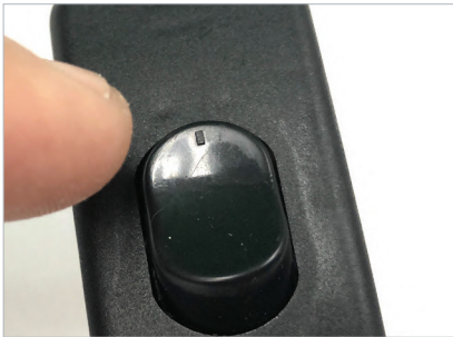
4. If the OBD2 extension cable is used, ensure the ON/OFF switch is in the ON position.
