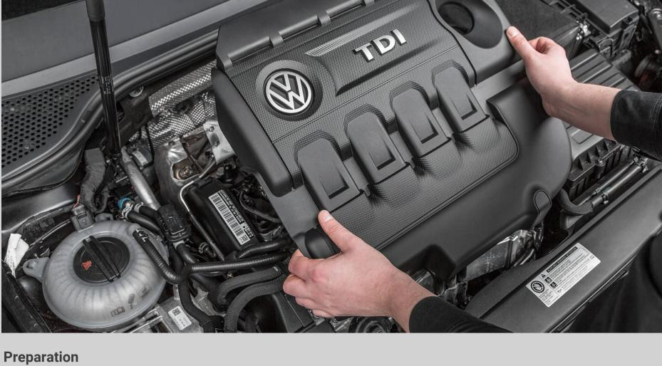
First, open the hood and remove the engine cover as shown in the example for the VW Passat (B8) 2.0 TDI with 110kW.
