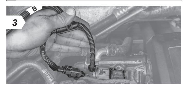
• Now connect the end of the RaceChip wiring harness marked "**B**" to the disconnected connector and the other end to the sensor.
