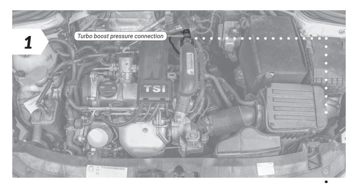
• First locate the turbo boost pressure sensor connection in your engine bay.
