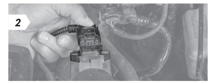
• Disconnect the plug from the turbo boost pressure sensor.
