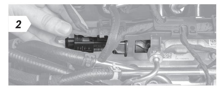
• Disconnect the plug from the common rail sensor.
