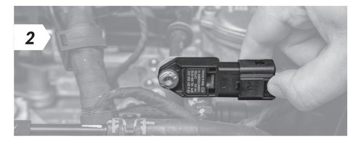
Disconnect the turbo boost pressure sensor
