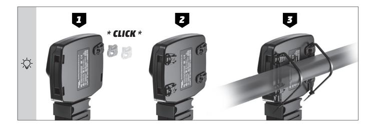
• If you need to remove the RaceChip at a later date, you can simply release the clips and do not have to cut any cable ties.
