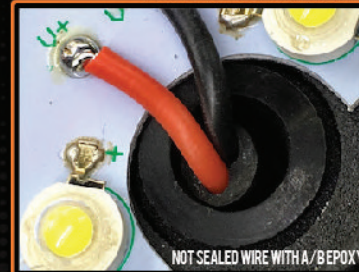
NOT WATERPROOF AND WEAK
