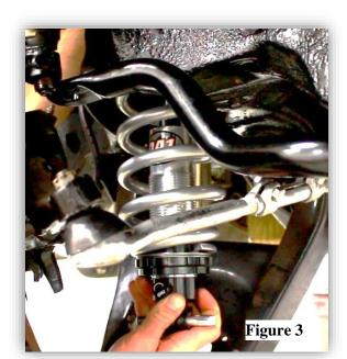
Mustang II: Install the supplied 7/16" or 1/2" lower shock bolts supplied. For Mx301 shocks, install a spacer on each side of the spherical bearing.
