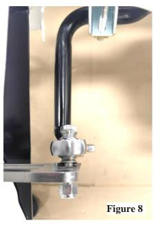
6. Attach one end of the assembled sleeve to the frame mount using two high misalignment spacers installed into the rod end. Fasten to frame mount using 3/8" x 2.5" bolts, with washer on the nylock nut side of the mount. The sway bar link will mount to the rear of the mount in the third hole from the top as a starting point. Torque to 31 lb. ft. *(Figure 8)*
