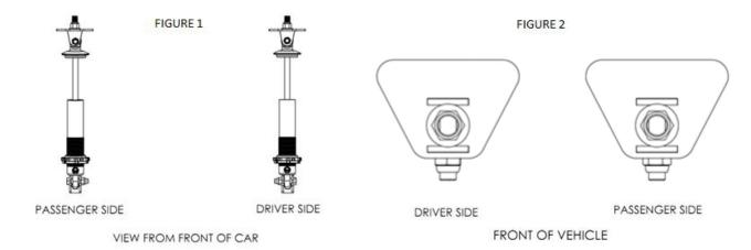
**Note:** Observe the installed orientation of the hardware (figure 1) in relation to the shock. The spring is not shown.
