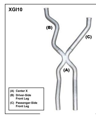
1. This three piece kit is designed to fit 1994-1996 GM Impala's. Measuring and cutting may be required. The x-pipe is designed to connect to your factory catalytic converters and run to the mufflers.
