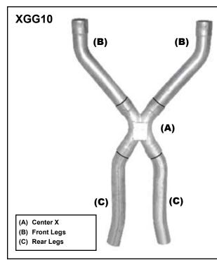
1. This three piece kit is produced to fit 1978-1988 GM G-bodies. Measuring and cutting may be required. The x-pipe is designed to connect to you collector reducers or down-pipes under the transmission cross-member.
