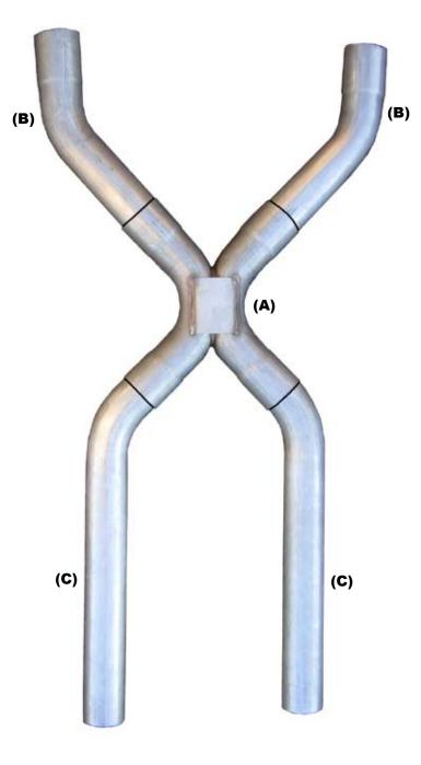
1. This five piece kit is a universal kit produced to fit many applications. Measuring and cutting will be required. The x-pipe is designed to connect to you collector reducers or down-pipes under the transmission cross-member.
