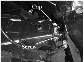
Under front bumper of the truck, unplug wiring harness from bulb, remove white cap. Then, remove factory adjustment screw using Phillips Screwdriver. (Spring will come off when screw is removed) Set parts aside, they will be used later for install.
