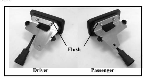
2. Install driver and passenger brackets on to fog lamp housing using supplied hardware. Verify that top edge of bracket is flush with edge of fog lamp housing. (Shown Above) Tighten hardware with Phillips Screwdriver.
