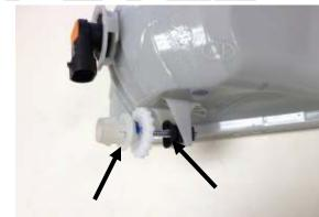
Remove adjustment screw and plastic adapter from factory fog lamp. (will be used in Step 5) Place fog lamp aside, this will not be used.
