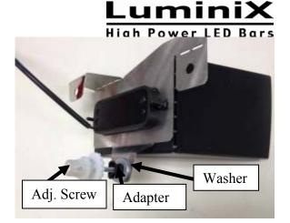
Place plastic adapter through 17/32" washer and into square hole on Putco fog lamp assembly as shown above. Thread adjustment screw into plastic adapter. (shown above)
