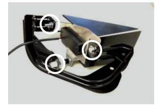
Snap adjustment screw clip back into factory bracket (removed in Step 3). Secure upper mounting locations with the 5/16" hardware.
