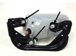
When factory fog lamp assembly is removed, use pliers to unclip (3) plastic clips (locations shown above) to remove bracket from factory fog lamp. Driver side is shown
