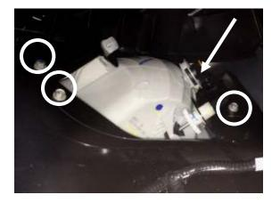
2. Remove (3) 10mm Bolts from factory fog lamp bracket. Unplug bulb from factory fog lamp and remove Lamp assembly from truck. **Passenger side is shown**. Repeat on Driver side. (wire loom clips my need to be removed to get fog lamp out)
