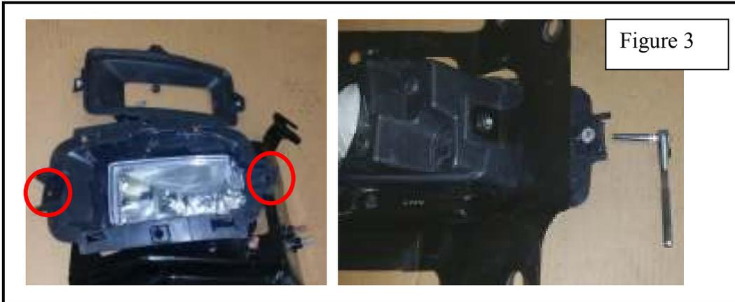
6. With the front cover removed the fog lamp can be removed from the front side. Use a Phillips screwdriver to push the fog lamp housing mounts out of the retaining clips. Refer to Figure 4.
