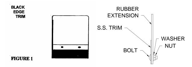
STEP 4: Attach the mud flap to the mud flap extension using 1/4" x 3/4" SS slot head bolts and nylon insert lock nuts. FIGURE 2
