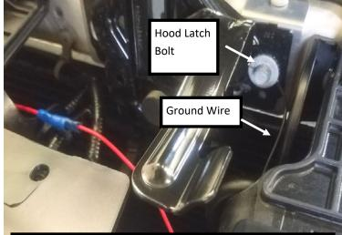
20. Connect Add-A-Fuse harness to red wire from LED emblem. Strip ~1/2" of insulation from black wire, and ground to chassis. For example, loosen (do not remove) the 10mm bolt holding hood latch enough to wrap black ground wire around bolt. Tighten bolt, making sure wire is secured.
