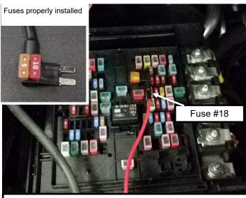
Remove Fuse #18 (10A fuse). Insert it in Add-A-Fuse tap and install provided 5A fuse on wire side of Add-A-Fuse tap, as pictured. Install assembly in Fuse #18 slot.
