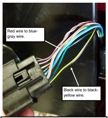
7. Using provided ScotchLoks, splice the wires into tail lamp harness. Connect the emblem red wire to the blue gray wire, and the emblem black wire to the black yellow wire.
