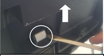
11. Using a flat head screwdriver, depress the clip while pulling the shutter system away from the grille. Repeat this process for (5) clips. The grille can now be separated from the shutter system.
