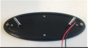
4. Install threaded rods and tighten by hand. Install the emblem on the tailgate using provided flange nuts. **BE CAREFUL NOT TO OVERTIGHTEN FASTENERS**.
