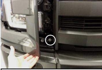
5. Remove (2) 8mm bolts securing lower grill to truck. Passenger side shown above. Repeat on driver side.
