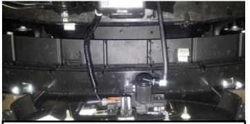
17. Reconnect any plugs for camera system and washer nozzle, if applicable. Feed LED emblem wires towards top of grille to finalize connections. Push grille into place, but do not install fasteners until emblem has been fully installed and tested.
