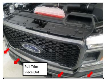
5. Starting from one wheel well, pull the bumper trim piece out to unclip the fasteners. Set the bumper trim piece aside.
