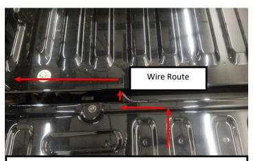
6. Feed LED emblem wires to driver's tail lamp harness. Follow existing harness coming out of tailgate. Route the wire under the vehicle, behind the bumper, and up into the tail lamp cavity. Protect the wire with split loom or abrasion resistant sleeving.
