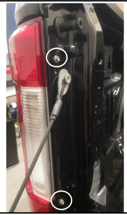
5. Remove (2) 8mm bolts from driver's tail lamp. Pull the tail lamp towards the rear bumper to disengage clips that secure it.
