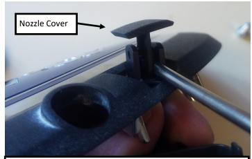
13. **Front camera equipped trucks:** Remove (3) T25 torx screws mounting camera assembly to emblem. Remove spray nozzle cover by gently prying arms with flat head screwdriver.
