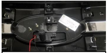
16. Install emblem onto grille with provided nuts. Tighten with 8mm wrench, being careful not to overtighten.
