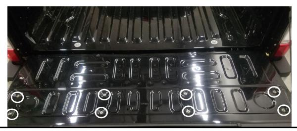
1. Lower tailgate and remove the eight T-30 screws from the access cover. Remove access cover.
