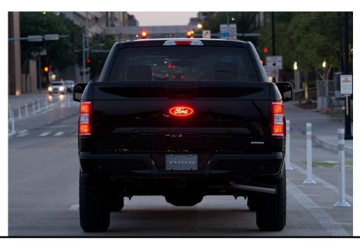
8. Test the emblem. It is tied to the running lamps and should be on when the Daytime Running Lamps or head lights are on. Zip-tie wires into place, making sure the wire is protected from pinch-points and sharp edges.
