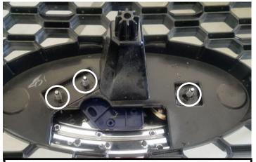
12. Remove (3) 10mm nuts holding emblem on. Disconnect any connectors, if camera is equipped.
