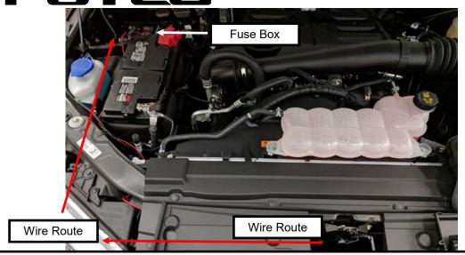
18. Connect the Add-A-Fuse tap to the LED emblem and route the wire to the fuse box. Be careful to avoid sharp edges and moving parts. Zip-tie wire in place when installation is complete.
